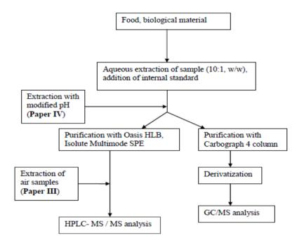
**Figure 3.** Summary LC-MS/MS-based method for measurement of acrylamide in food (Eriksson 2005)
